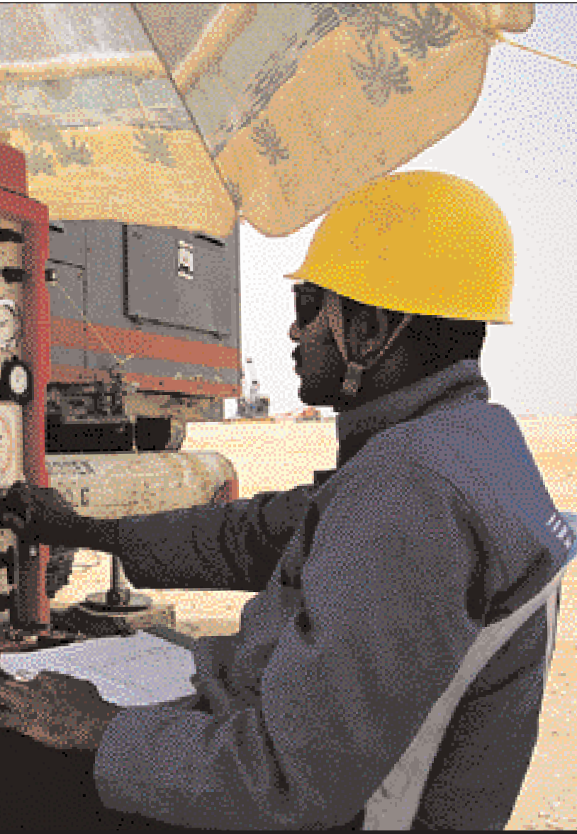
THE MARS PROCESS (MENARD AUTOMATIC RELEASE SYSTEM) optimizes the energy from ground compaction by eliminating energy loss from braking or friction.
